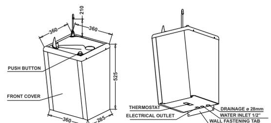
Installation by means of three basic connection points.
